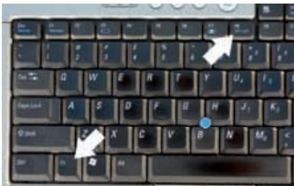
3. The laptop may detect automatically the external device. If not, on most laptops one uses the 'Fn' key and a key marked 'CRT/LCD' (and/or with a little picture of a monitor) to turn the display on manually.
