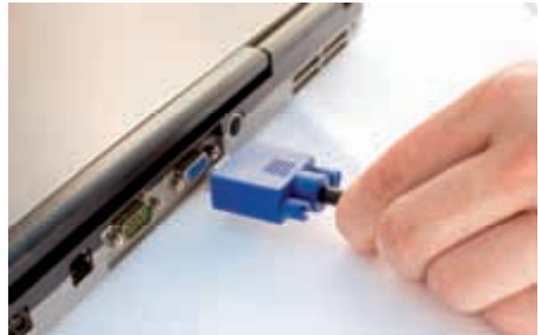
2. Plug the cable from the PC projector, or other external display device, into the matching port on the laptop. Switch on the external display device and switch on the laptop.
